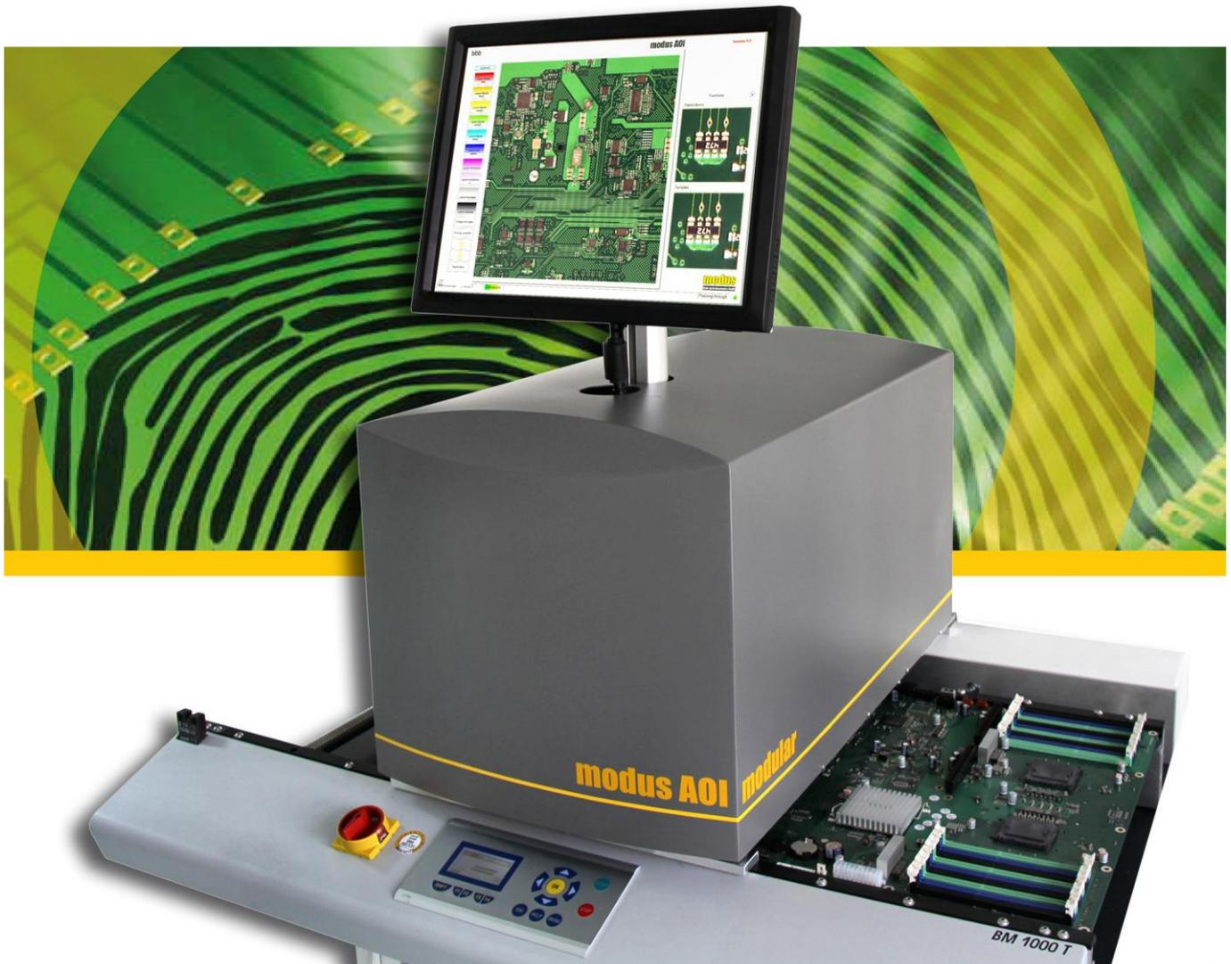
The nearly maintenance-free modusAOI modular was specially developed for transport conveyor modules in production lines. Existing lines can easily be retrofitted with the scan unit, which inspects the test item without interruption while it is being conveyed to the next processing station. The scanner, sensors and computer are integrated in the housing.
